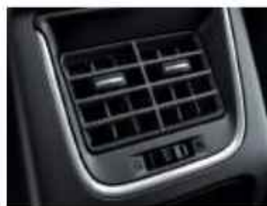
REAR AC VENT
